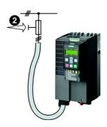
After it has been switched on, the frequency inverter copies its settings to the memory card.
