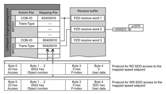
Figure 7-19 Access to the process data
