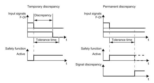
Figure 8-33 Tolerance regarding discrepancy
