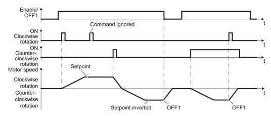
Figure 8-6 Three-wire control, method 1
