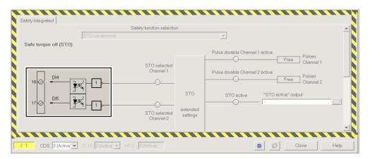
Figure 8-37 Example: Assignment of digital inputs DI 4 and DI 5 with STO
