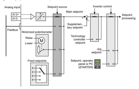
Figure 8-11 Setpoint sources for the converter
