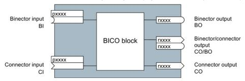
Figure A-7 Symbols for binector and connector inputs and outputs
