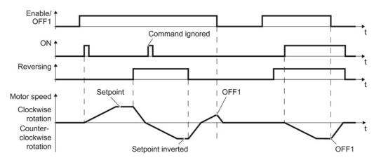
Figure 8-7 Three-wire control, method 2
