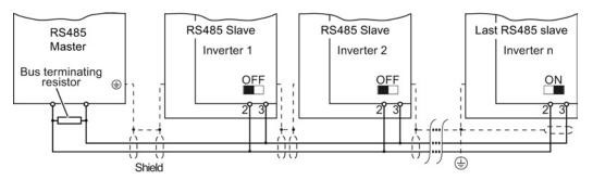
Figure 7-8 Communication network via RS485
