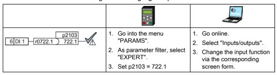
You have interconnected digital input DI 1 with the command to acknowledge faults.
