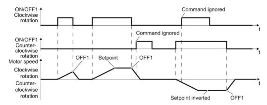
Figure 8-4 Two-wire control, method 2
