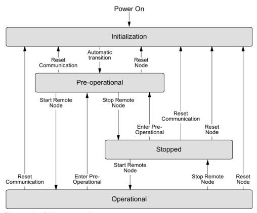
Figure 7-18 CANopen state diagram
