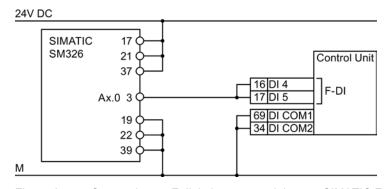
Figure A-14 Connecting an F digital output module, e.g. SIMATIC F digital output module
