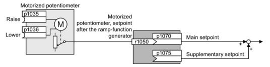
Figure 8-14 Motorized potentiometer as setpoint source
