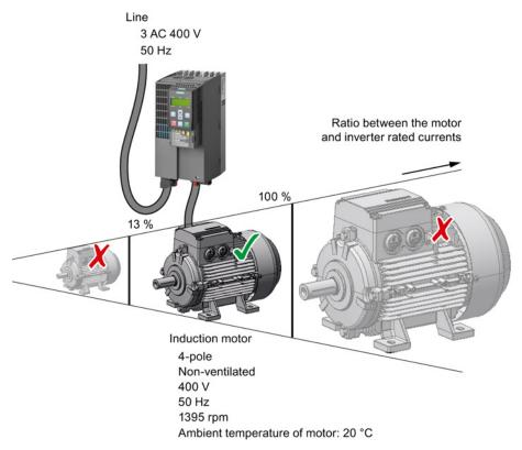
Figure 5-2 Motor data factory settings
