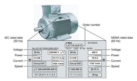
Figure 5-1 Motor data of the rating plate
