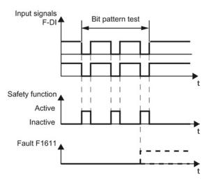
Figure 8-34 Inverter response to a bit pattern test
