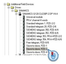
2. With a double-click, open the dialog box to make additional settings for the direct data exchange.
