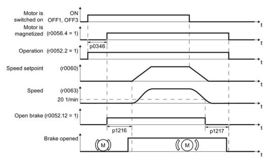
Figure 8-27 Controlling the motor holding brake when the motor is switched on and off
