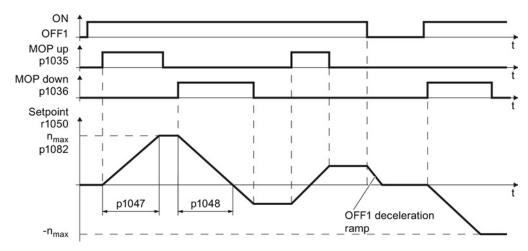
Figure 8-15 Function chart of motorized potentiometer
