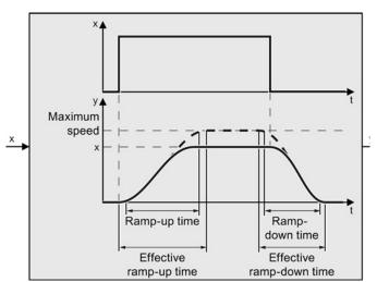
Table 8- 20 Additional parameters to set the extended ramp-function generator
