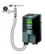
After it has been switched on, the frequency inverter copies its settings to the memory card.
