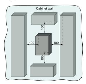
Figure 4-3 Distances of line reactors to other equipment [mm]
