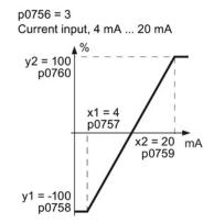
Figure 6-3 Examples for scaling characteristics
