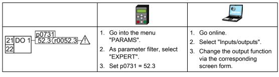
You have interconnected digital output DO 1 with the fault message.
