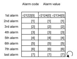
Figure 11-3 Complete alarm buffer
