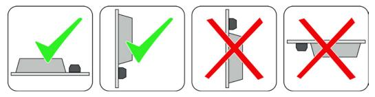
Figure 4-4 Permissible mounting orientation of the braking resistor
