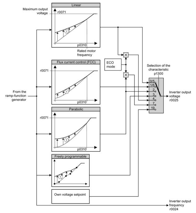
① The voltage boost of the characteristic improves motor behavior at low speeds. The voltage boost is effective for frequencies < rated frequency
