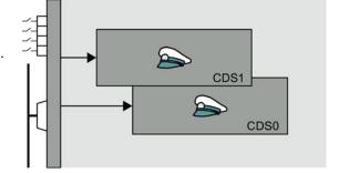
You select the command data set using parameter p0810. To do this, you must interconnect parameter p0810 with a control command of your choice, e.g. a digital input.
