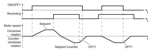
Figure 8-3 Two-wire control, method 1
