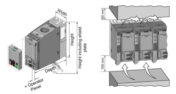
Figure 4-2 Dimensions and minimum spacing to other devices
