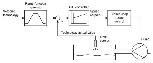
Figure 8-31 Example: technology controller as a level controller
