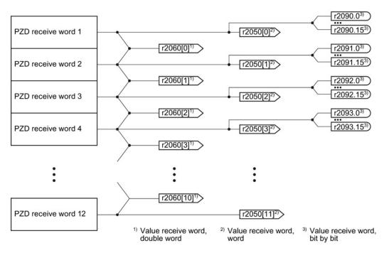
Figure 7-4 Interconnection of the receive words
