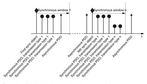
Figure 7-21 Principle of synchronous and asynchronous transmission
