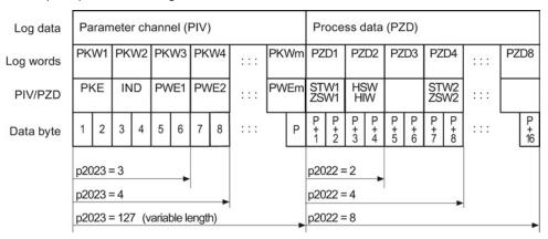
Figure 7-10 USS telegram - user data structure
