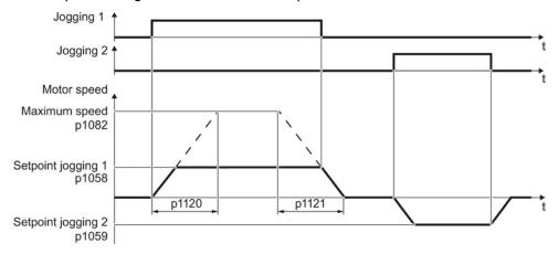
Figure 8-8 Behavior of the motor when "jogging"
