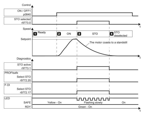
Figure 8-39 Acceptance test for STO (basic functions)
