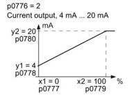
Figure 6-5 Examples for scaling characteristics
