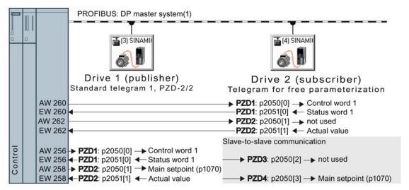
Figure A-11 Communication with the higher-level controller and between the drives with direct data exchange
