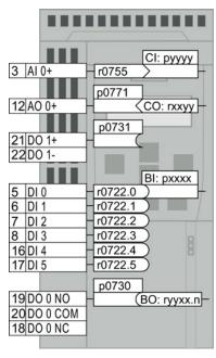
Figure 6-1 Internal connection of the inputs and outputs
