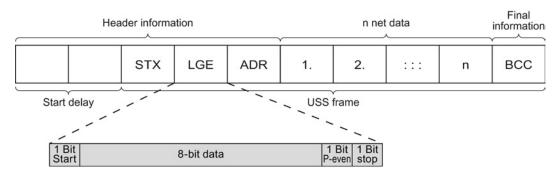
Figure 7-9 Structure of a USS telegram
