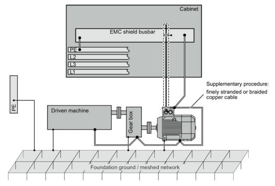
Figure 4-7 Additional high-frequency bonding of the drive system
