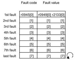
Figure 11-7 Complete fault buffer
