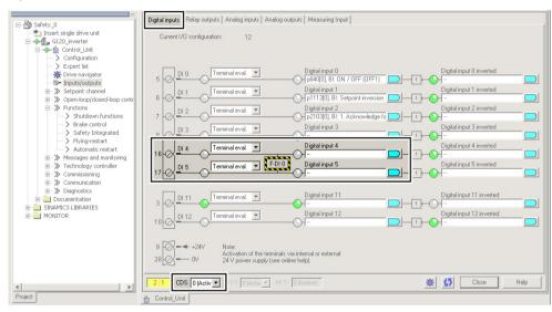
Figure 8-38 Remove pre-assignment of digital inputs DI 4 and DI 5
