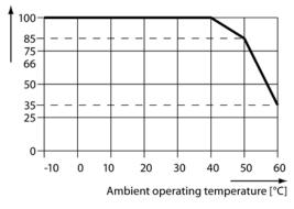
Figure 12-2 Temperature derating
