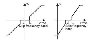
Figure 6-4 Skip frequency band of the analog input
