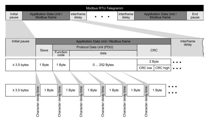
Figure 7-17 Modbus with delay times
