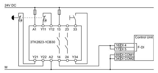
Figure A-13 Connecting a safety relay, e.g. SIRIUS 3TK28
