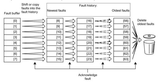
Figure 11-8 Fault history after acknowledging the faults
