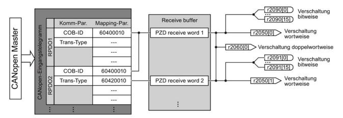
Structure of the mapping parameter using the control word in the predefined connections set as an example
