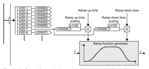
Figure 8-19 Example for changing the ramp-function generator times in operation
