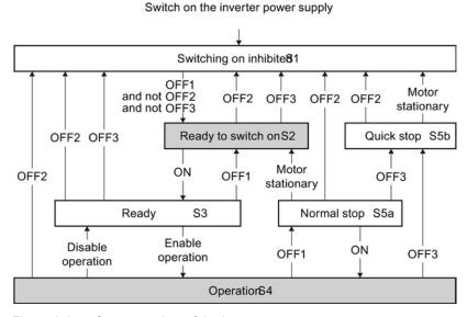
Figure 8-2 State overview of the inverter
