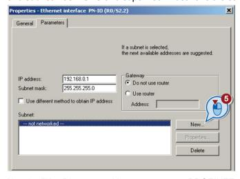
5. Use the "New" button to either create a new PROFINET subnet or select an existing one.
