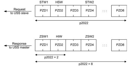
Figure 7-14 Process data channel
