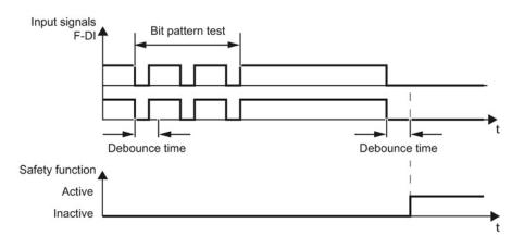
Figure 8-35 Filter for suppressing temporary signal changes
