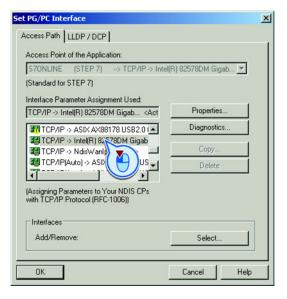
You have allocated your computer the IP address and the address of the subnet mask, and defined the PC interface via which STARTER goes online with the inverter.
