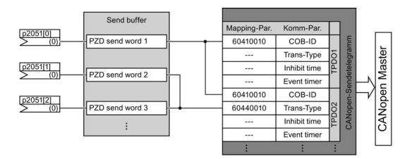
Structure of the communication parameter using the status word in the predefined connections set as an example
