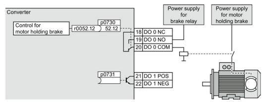
Figure 8-26 Simplified diagram of motor holding brake connected to DO 0 of the converter
