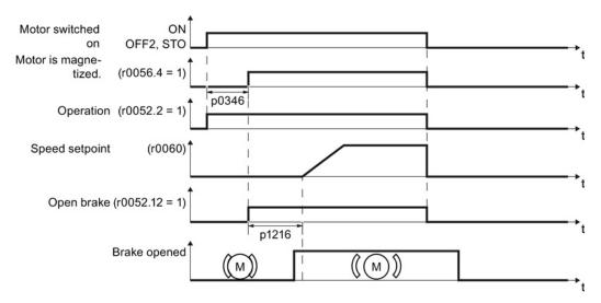
Figure 8-28 Controlling the motor holding brake after an OFF2 command or selecting STO
