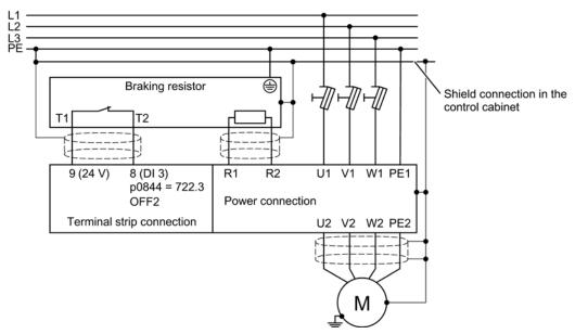
Figure 8-25 Braking resistor connections (Example: temperature monitoring via DI 3)
