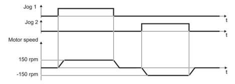
Figure 5-4 Jogging the motor in the factory setting
