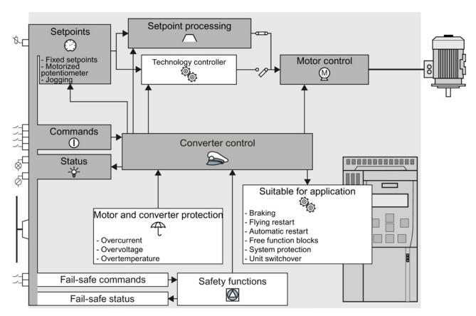
Figure 8-1 Overview of inverter functions
