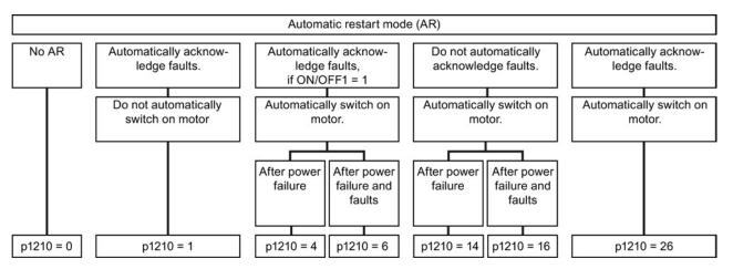
Figure 8-29 Selecting the automatic restart mode
