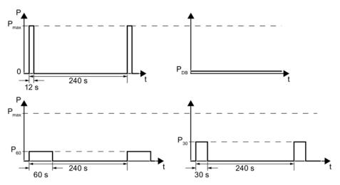
Figure 12-4 Pulse power, rated power and duty cycle examples of the braking resistor
