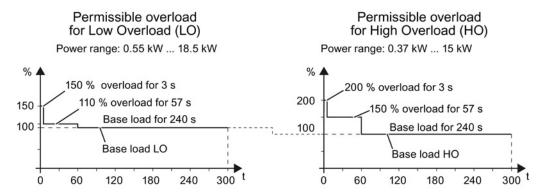
Figure 12-1 Duty cycles, "High Overload" and "Low Overload"
