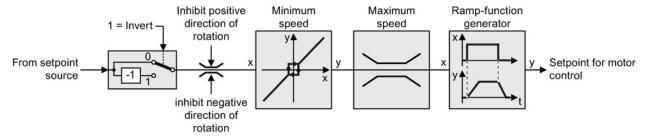
Figure 8-18 Setpoint processing in the inverter
