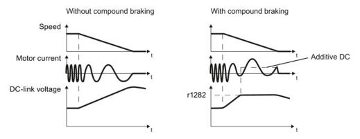
Figure 8-23 Motor brakes with and without active compound braking
