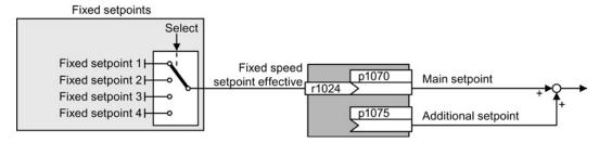
Figure 8-16 Fixed speeds as setpoint source
