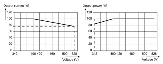
Figure 12-3 Current and Power derating required according to input voltage
