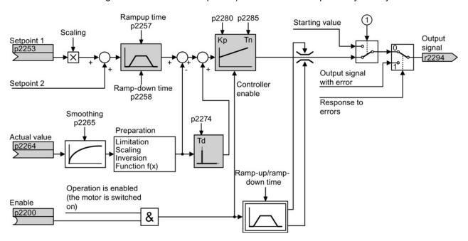
Figure 8-32 Simplified representation of the technology controller
