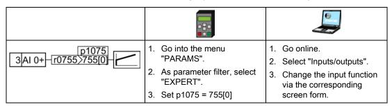
You have interconnected the analog input with the additional setpoint.
