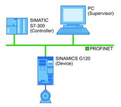
Figure 7-1 Example: PROFINET in a line topology
