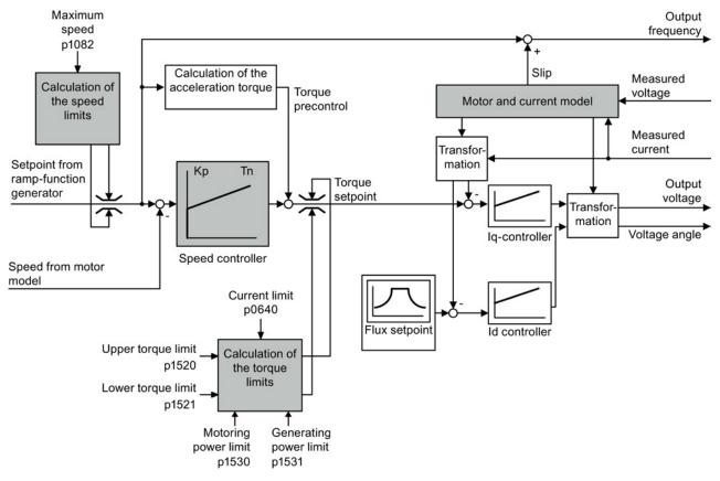
Figure 8-21 Simplified function diagram of sensorless vector control
