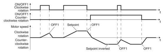
Figure 8-5 Two-wire control, method 3
