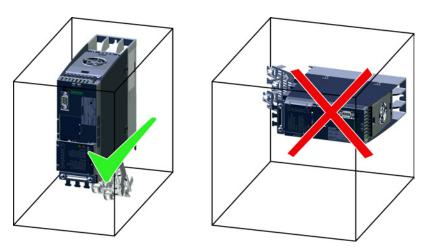
Figure 4-1 The converter must not be installed horizontally.
