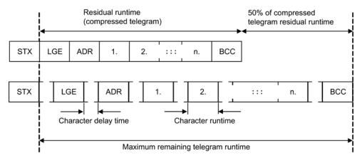
Figure 7-15 Telegram runtime as the sum of the residual runtime and character delay times
