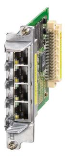
Figure 4-29 Communication Board Ethernet CBE20
