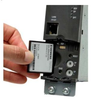
Figure 4-17 CompactFlash card slot
