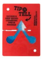
Figure 3-4 Tilt indicator tripped
