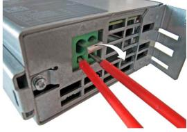
Terminal X530 with connector jumper
