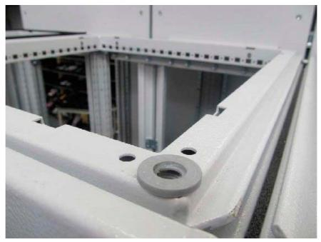
Figure 3-18 Attaching the washers
