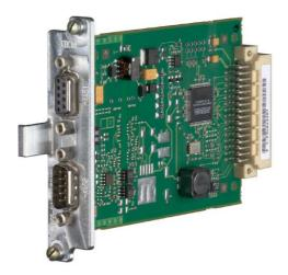
Figure 4-27 CAN CBC10 Communication Board
