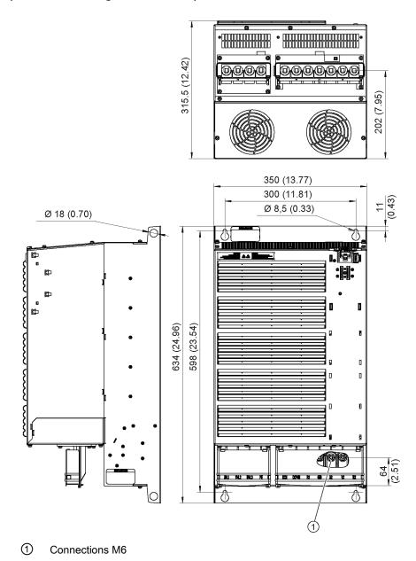
Figure 4-14 Dimension drawing, PM340 Power Module, frame size FSF (without integrated line filter); all dimensions in mm and (inches)
