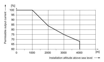
Figure 4-46 Output current as a function of the installation altitude
