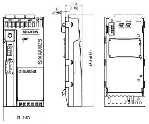
Figure 7-18 Dimension drawing of Control Unit Adapter CUA31, all data in mm and (inches)
