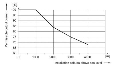
Figure 4-26 Output current as a function of the installation altitude
