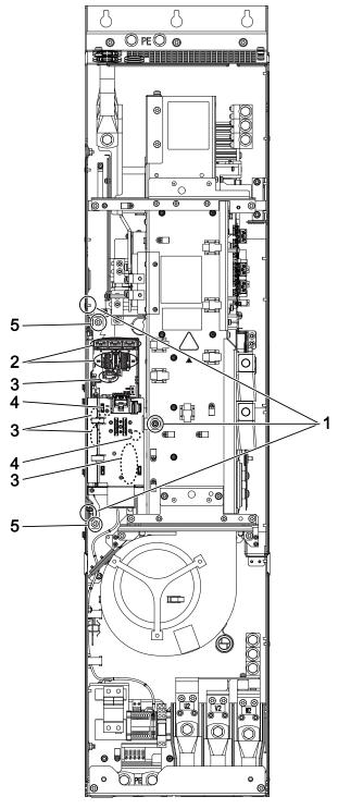
Figure 12-8 Replacing the Control Interface Module, Power Module, frame size FX
