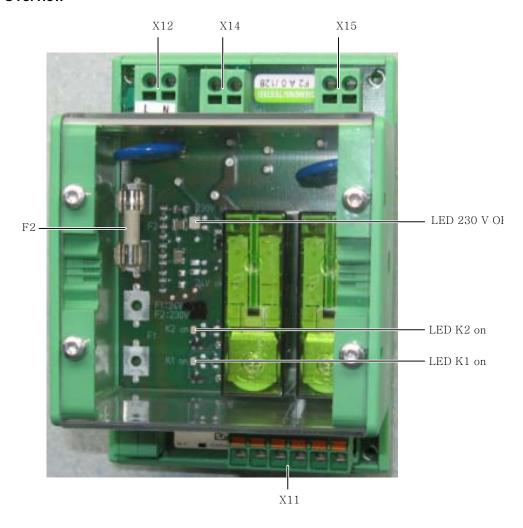
Figure 8-14 Interface overview, Safe Brake Adapter 230 V AC
