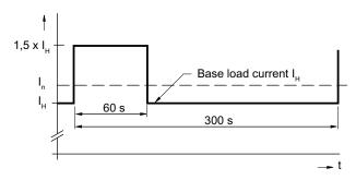
Figure 4-41 Duty cycle with 60 s overload with a duty cycle duration of 300 s
