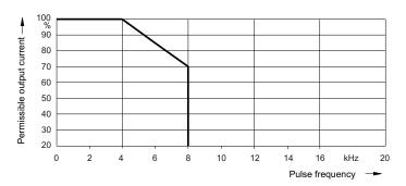
Figure 4-24 Frame size FSF: Output current as a function of the pulse frequency
