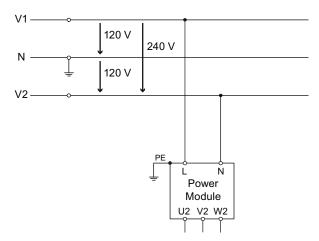
Figure 3-21 Direct operation on single phase grounded midpoint line system configurations
