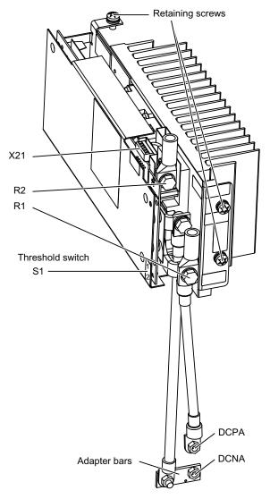
Figure 5-6 Braking Module for Power Module, frame size FX
