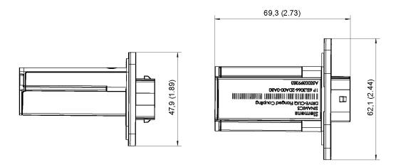
Figure 9-3 Dimension drawing of the DRIVE-CLiQ cabinet bushing RJ45, all dimensions in mm and (inches)
