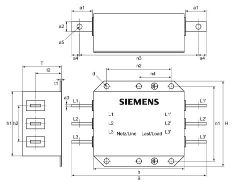
Figure 3-4 Dimension drawing, line filter
