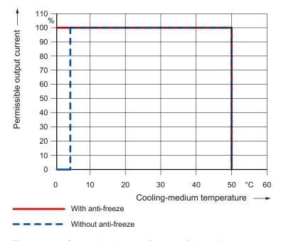
Figure 4-49 Current derating as a function of the ambient temperature
