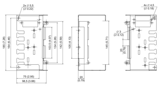
Figure 9-16 Dimension drawing, screening kit, frame size FSC, all data in mm (inches)
