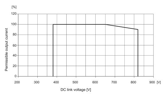
Figure 4-48 Current derating as a function of the DC-link voltage
