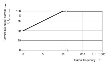
Figure 4-47 Output current as a function of the output frequency
