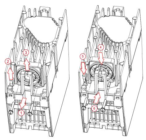
Figure 12-1 PM340 fan replacement, frame size FSA
