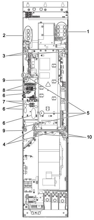
Figure 12-7 Replacing the Powerblock, Power Module, frame size GX
