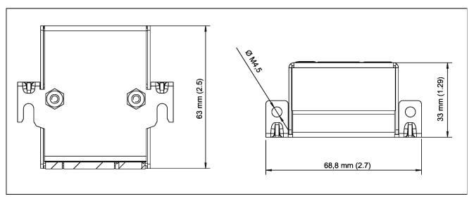
Figure 8-11 Dimension drawing of Safe Brake Relay, all data in mm and (inches)
