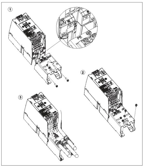
Figure 9-23 Mounting: Screening kit on a Power Module (FSA)
