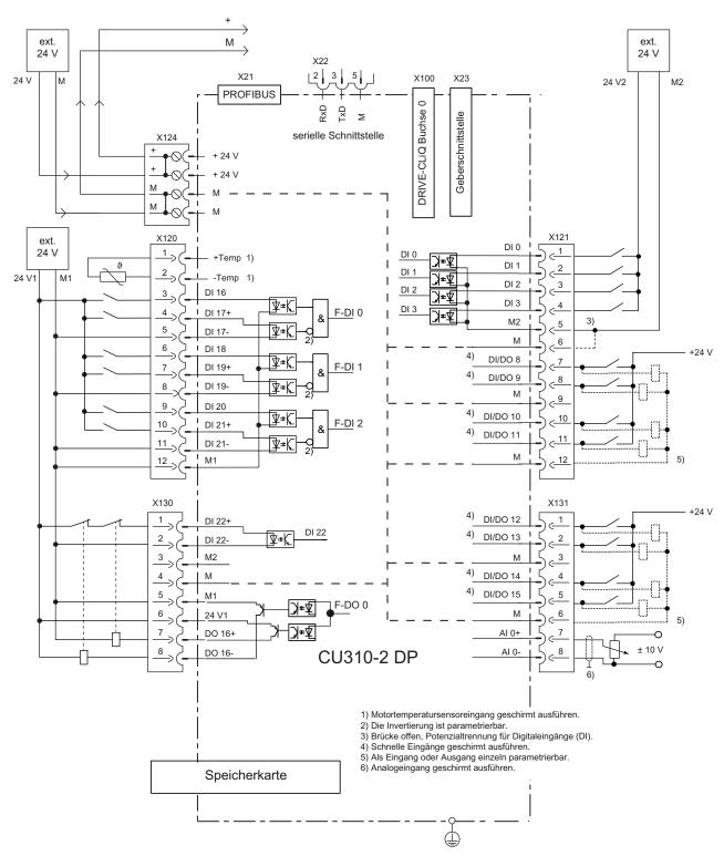
Figure 7-14 Connection example, CU310-2 DP with safety function
