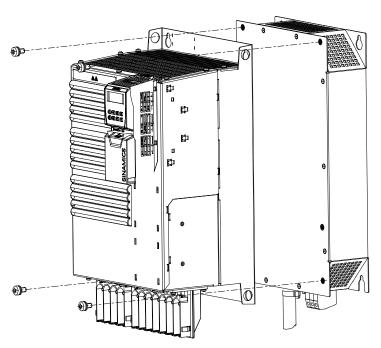
Figure 3-16 Mounting the PM340 with a line reactor, using frame size FSD as an example
