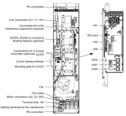
Figure 4-50 Power Module, frame size FX
