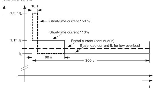
Figure 4-57 Characteristic: Low overload
