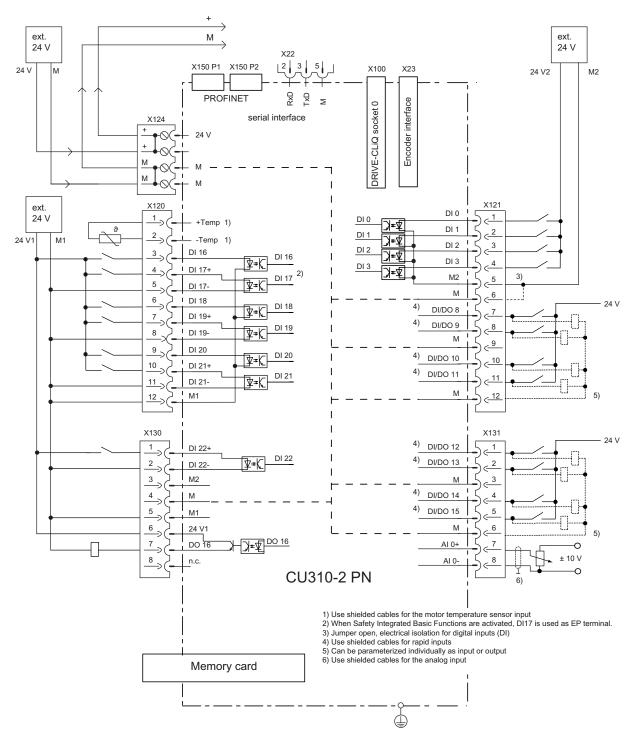
Figure 7-6 Connection example, CU310-2 PN without safety function
