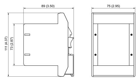
Figure 8-16 Dimension drawing of Safe Brake Adapter, all data in mm and (inches)
