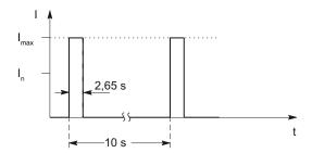
Figure 4-38 Duty cycle without initial load (for servo drives)
