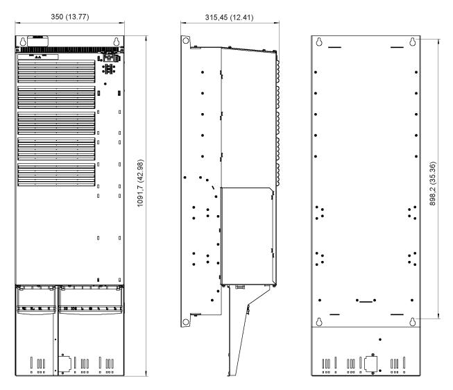
Figure 9-22 Dimension drawing, PM340 Power Module with screening kit, frame size FSF with integrated line filter, all dimensions in mm (inches)
