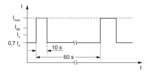
Figure 4-40 Duty cycle with initial load (for servo drives)
