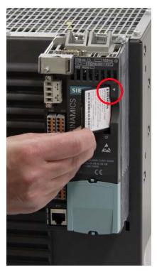
Figure 7-5 CU310-2 PN Inserting the memory card
