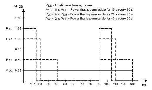
Figure 5-11 Duty cycle for braking resistors
