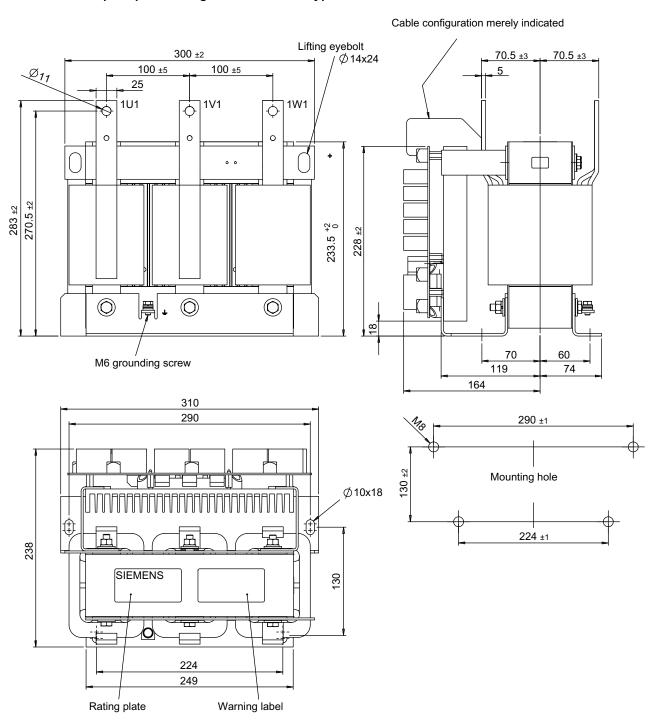
Figure 6-22 Dimension drawing of dv/dt filter compact plus Voltage Peak Limiter, type 1
