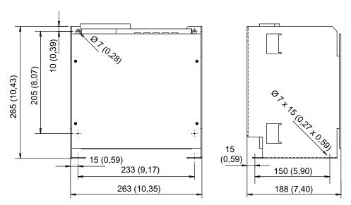
Figure 6-17 Dimension drawing of the voltage peak limiter, type 1
