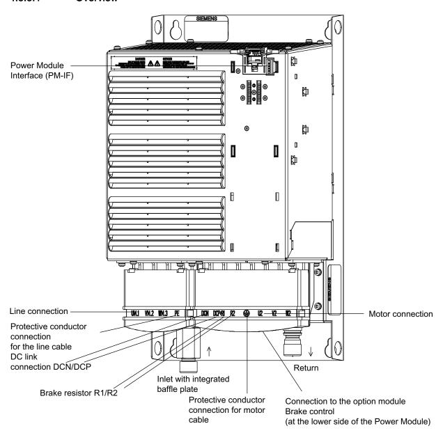
Figure 4-29 Liquid Cooled Power Module PM340 (Example: Frame size FSD)
