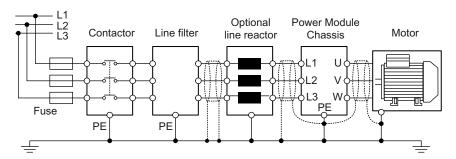
Figure 3-2 Example of a chassis line connection
