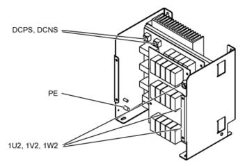
Figure 6-13 Interface overview, voltage peak limiter, type 1
