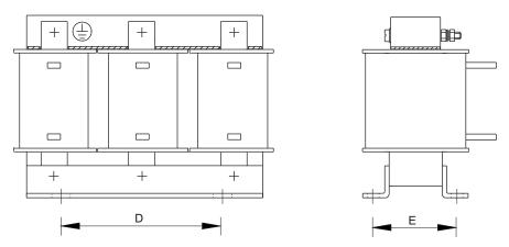
Figure 3-13 Mounting dimensions of line reactor, frame size FSF
