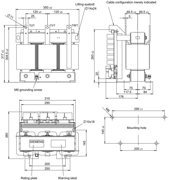
Figure 6-23 Dimension drawing of dv/dt filter compact plus Voltage Peak Limiter, type 2
