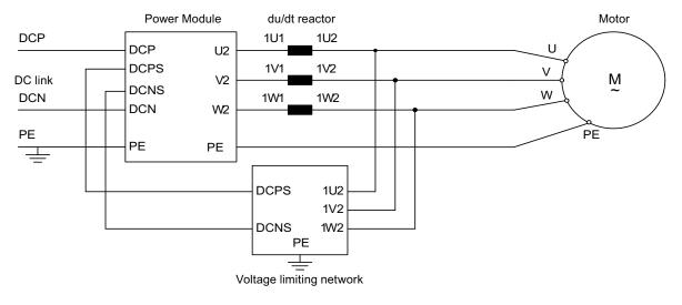
Figure 6-15 Connecting the du/dt filter plus Voltage Peak Limiter
