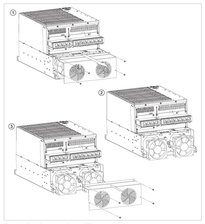
Figure 12-4 PM340 fan replacement, frame size FSF
