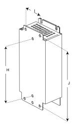
Figure 6-6 Mounting dimensions of motor reactor, frame size FSA
