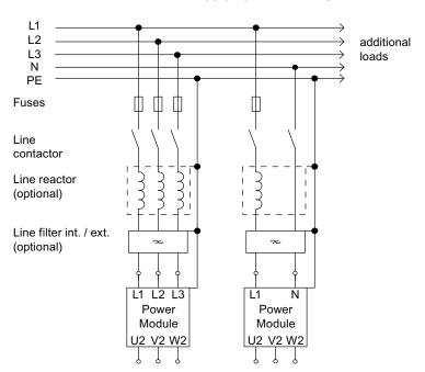
Figure 3-20 Direct operation on the line supply
