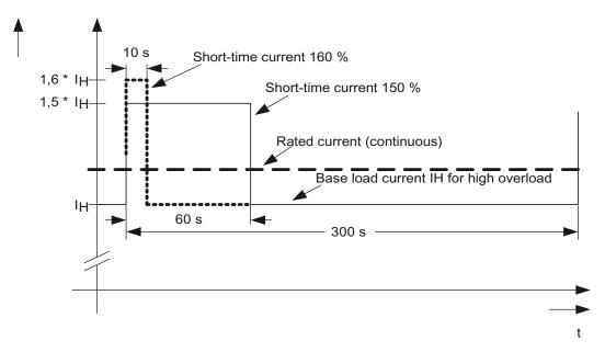
Figure 4-58 Characteristic: High overload
