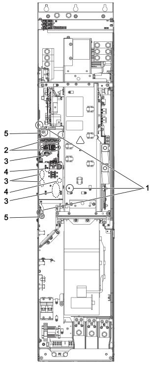
Figure 12-9 Replacing the Control Interface Module, Power Module, frame size GX
