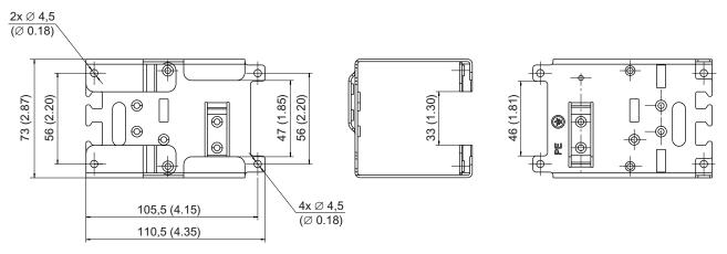
Figure 9-14 Dimension drawing, screening kit, frame size FSA, all data in mm (inches)
