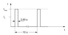
Figure 4-18 Duty cycle without initial load (for servo drives)
