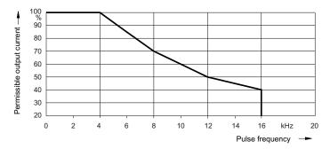
Figure 4-43 Frame sizes FSD and FSE: Output current as a function of the pulse frequency
