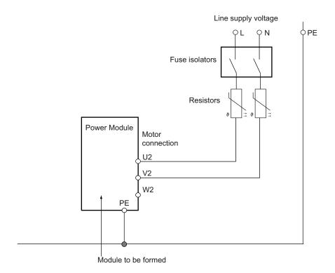
Figure 12-14 Forming circuit for 1-ph AC Power Modules with resistors
