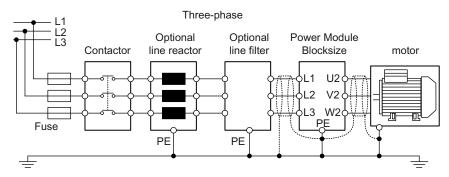
Figure 3-1 Example of a blocksize line connection for Power Modules with no integrated line filter
