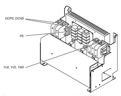
Figure 6-14 Interface overview, voltage peak limiter, type 2
