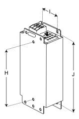
Figure 3-10 Mounting dimensions of line reactor, frame size FSA
