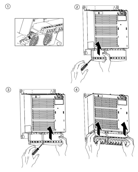
Figure 4-36 Access to the line and motor terminals for Liquid Cooled Power Modules
