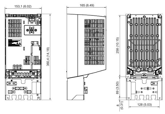
Figure 9-18 Dimension drawing, PM340 Power Module with screening kit, frame size FSB, dimensions in mm (inches)
