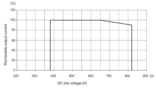
Figure 4-28 Current derating as a function of the DC-link voltage
