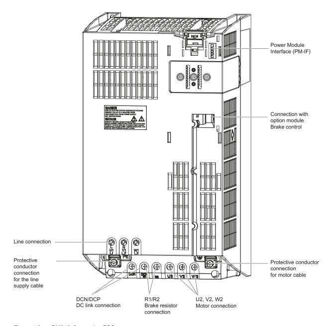
Figure 4-3 PM340, frame size FSC
