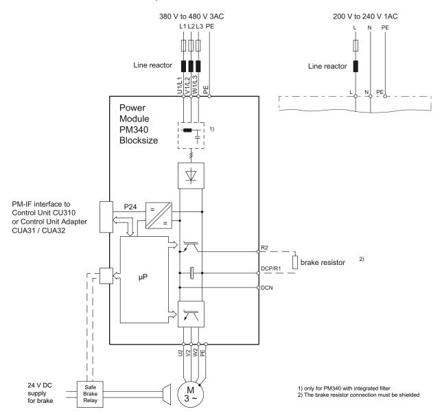
Figure 4-7 PM340 connection example
