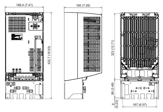
Figure 9-19 Dimension drawing, PM340 Power Module with screening kit, frame size FSC, dimensions in mm (inches)
