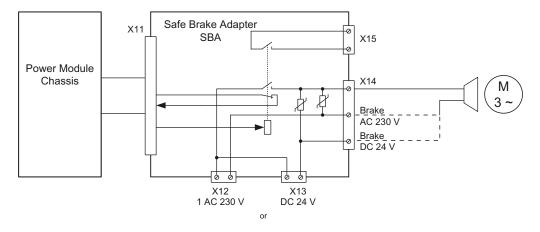
Figure 8-15 Connection example for a Safe Brake Adapter
