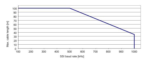
Figure 7-11 Maximum cable length as a function of the SSI baud rate for SSI encoders
