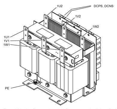
Figure 6-20 Interface overview, dv/dt filter compact plus Voltage Peak Limiter, type 2
