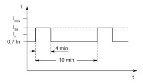
Figure 4-39 S6 duty cycle with initial load (for servo drives)
