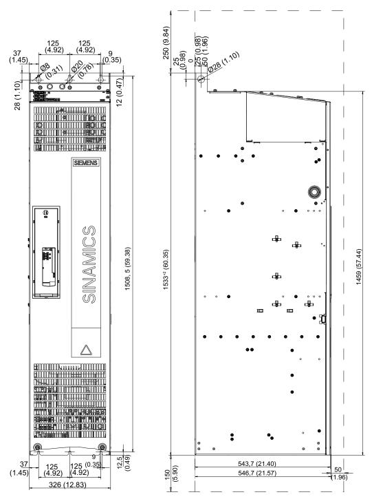
Figure 4-54 Dimension drawing Power Module, frame size GX
