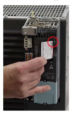
Figure 7-12 CU310-2 DP Inserting the memory card
