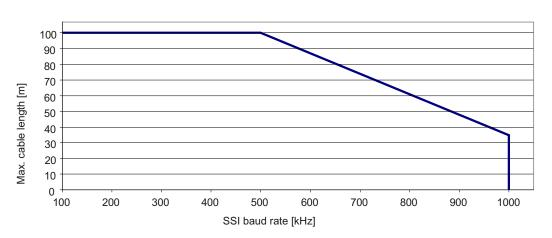
Figure 7-4 Maximum cable length as a function of the SSI baud rate for SSI encoders
