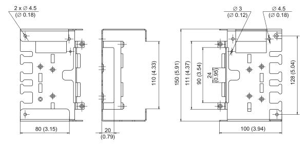
Figure 9-15 Dimension drawing, screening kit, frame size FSB, all data in mm (inches)
