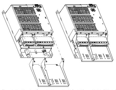
Figure 9-28 Mounting: Screening kit on a Liquid Cooled Power Module PM340, frame sizes FSD / FSE
