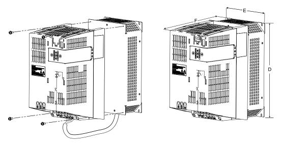
Figure 6-9 Mounting Power Modules and motor reactors, frame sizes FSB / FSC
