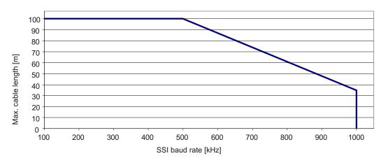
Figure 8-8 Maximum cable length as a function of the SSI baud rate for SSI encoders
