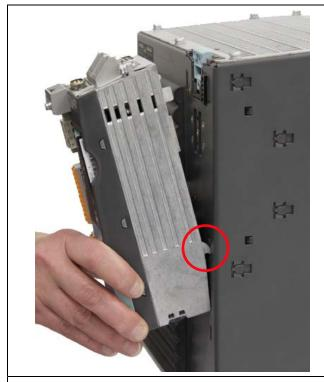
Placing the CU310-2 PN on the PM340
