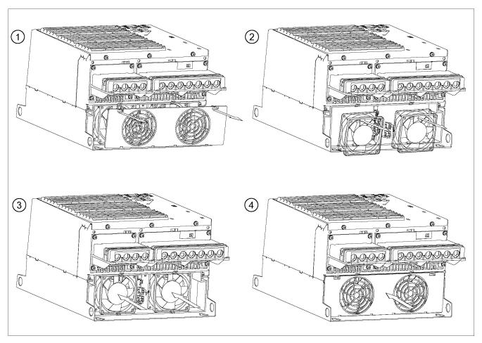
Figure 12-3 PM340 fan replacement, frame sizes FSD/FSE
