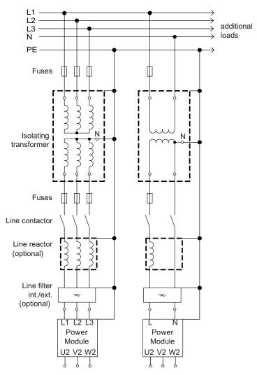
Figure 3-23 Isolating transformer
