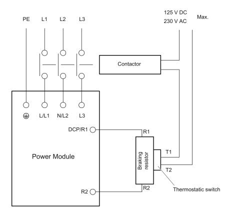
Figure 5-2 Connecting the thermostatic switch on the braking resistor to a contactor
