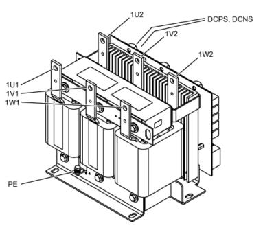
Figure 6-19 Interface overview, dv/dt filter compact plus Voltage Peak Limiter, type 1
