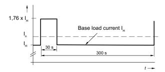
Figure 4-42 Duty cycle with 30 s overload with a duty cycle duration of 300 s
