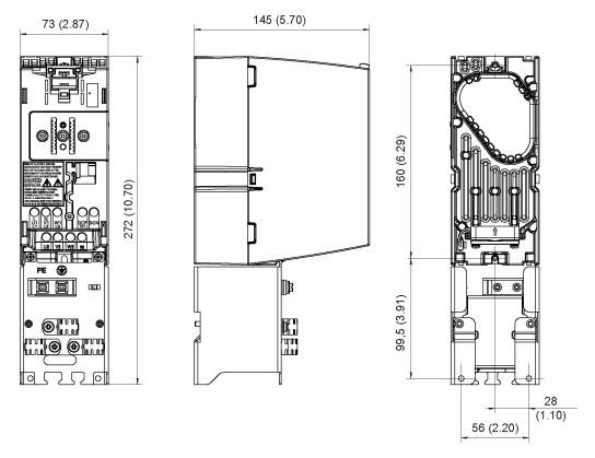
Figure 9-17 Dimension drawing, PM340 Power Module with screening kit, frame size FSA, dimensions in mm (inches)
