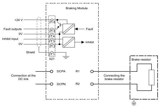
Figure 5-8 Example connection of Braking Module
