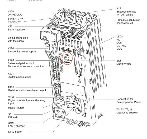
Figure 7-2 CU310-2 PN overview of interfaces
