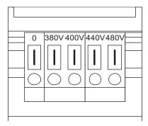
Figure 4-55 Setting terminals for the fan transformers
