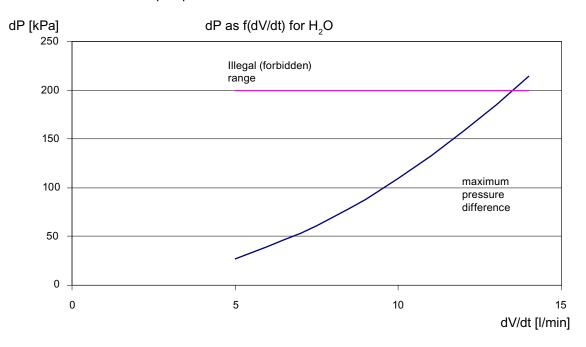
Figure 11-3 Pressure difference as a function of volumetric flow
