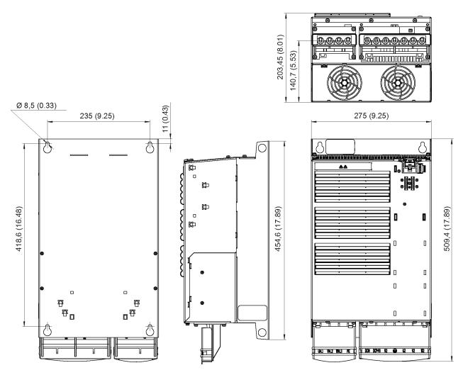
Figure 4-11 Dimension drawing, PM340 Power Module, frame size FSD (with integrated line filter); all dimensions in mm and (inches)
