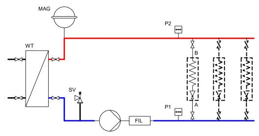
Figure 11-1 Example of a closed cooling circuit
