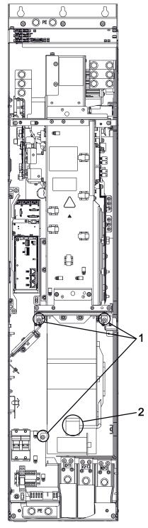
Figure 12-11 Replacing the fan, Power Module, frame size GX
