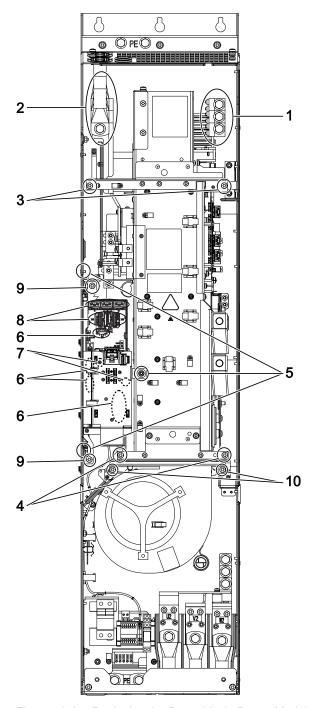
Figure 12-6 Replacing the Powerblock, Power Module, frame size FX
