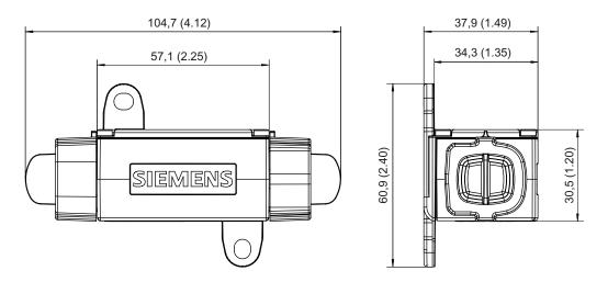
Figure 9-11 Dimension drawing of the DRIVE-CLiQ coupling, all dimensions in mm and (inches)
