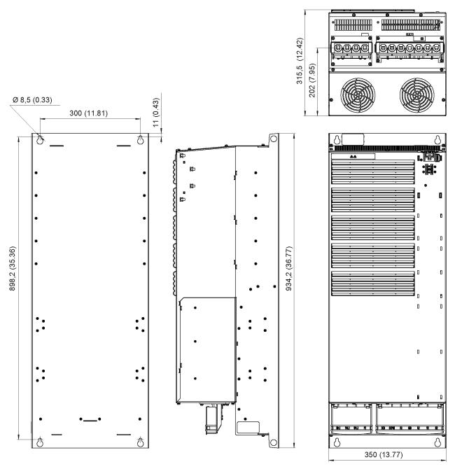
Figure 4-15 Dimension drawing, PM340 Power Module, frame size FSF (with integrated line filter); all dimensions in mm and (inches)
