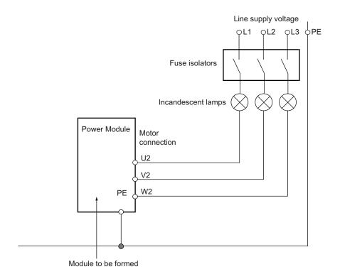
Figure 12-12 Forming circuit for 3-ph AC Power Modules with incandescent lamps
