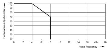
Figure 4-44 Frame size FSF: Output current as a function of the pulse frequency
