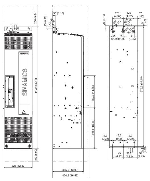
Figure 4-53 Dimension drawing Power Module, frame size FX
