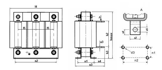
Figure 6-8 Mounting dimensions, motor reactors, frame sizes FSD / FSE / FSF
