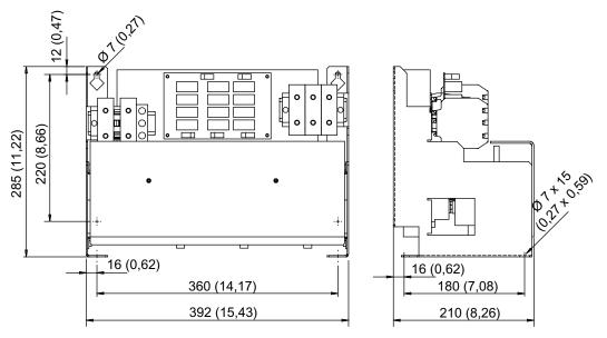
Figure 6-18 Dimension drawing of the voltage peak limiter, type 2
