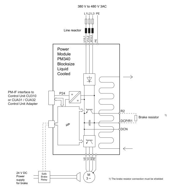
Figure 4-30 Connection example Power Module PM340 Liquid Cooled, 3 AC 380 V to 480 V
