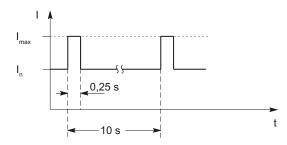
Figure 4-37 Duty cycle with initial load (for servo drives)
