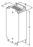
Figure 6-1 Dimension drawing, motor reactor, frame size FSA
