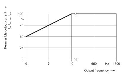
Figure 4-27 Output current as a function of the output frequency
