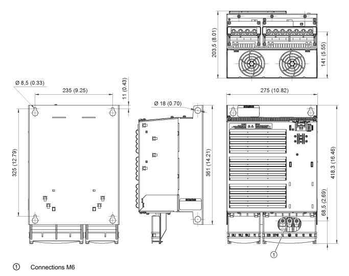
Figure 4-10 Dimension drawing, PM340 Power Module, frame size FSD (without integrated line filter); all dimensions in mm and (inches)
