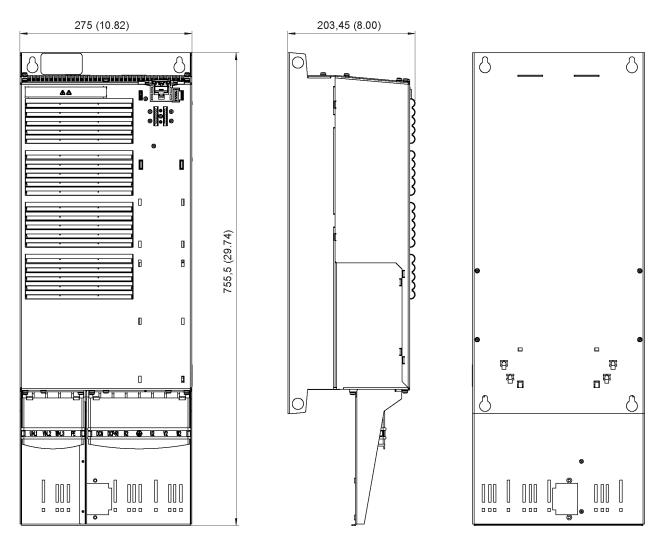
Figure 9-21 Dimension drawing, PM340 Power Module with screening kit, frame size FSE with integrated line filter, dimensions in mm (inches)
