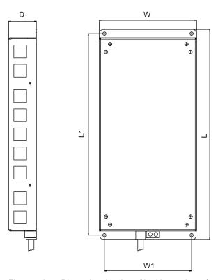
Figure 5-3  $\,\,$  Dimension drawing of braking resistor, frame sizes FSA / FSB
