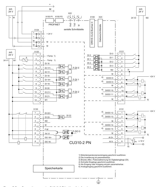
Figure 7-7 Connection example, CU310-2 PN with safety function
