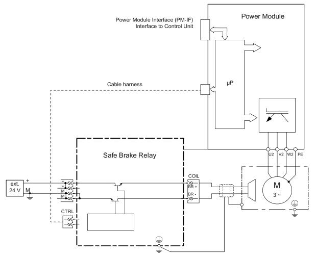
Figure 8-10 Safe Brake Relay connection example
