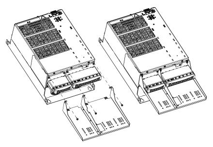
Figure 9-26 Mounting: Screening kit on a Power Module (FSD/FSE)
