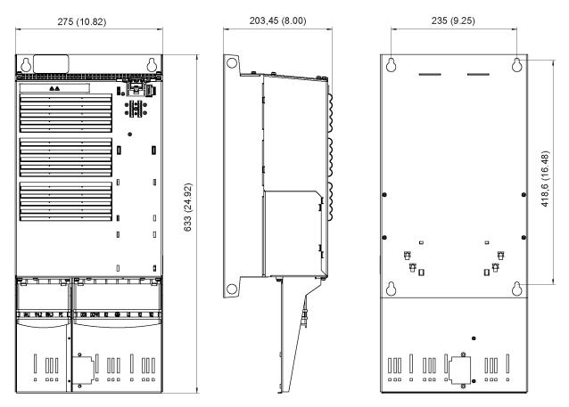
Figure 9-20 Dimension drawing, PM340 Power Module with screening kit, frame size FSD with integrated line filter, dimensions in mm (inches)
