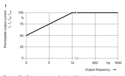
Figure 4-59 Output current as a function of the output frequency
