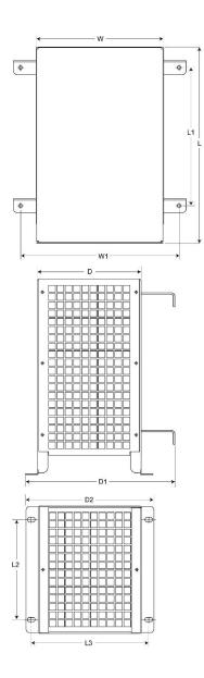
Figure 5-4 Dimension drawing of braking resistor, frame sizes FSC / FSD / FSE / FSF
