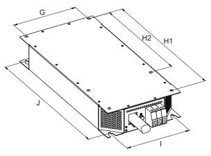
Figure 3-12 Mounting dimensions of line reactor, frame sizes FSD and FSE
