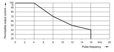
Figure 4-23 Frame sizes FSA to FSE: Output current as a function of the pulse frequency
