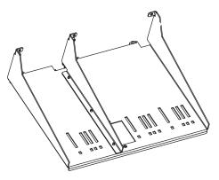
Figure 9-13 Screening kit for attachment to a Power Module, frame size FSD/FSE
