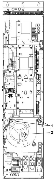
Figure 12-10 Replacing the fan, Power Module, frame size FX
