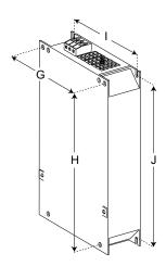
Figure 3-11 Mounting dimensions of line reactor, frame sizes FSB and FSC
