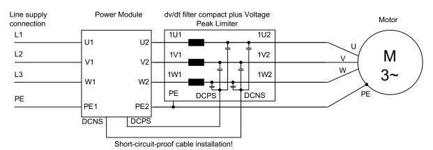
Figure 6-21 Connecting the dv/dt filter compact plus Voltage Peak Limiter
