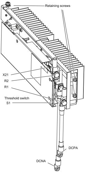
Figure 5-7 Braking Module for Power Module, frame size GX
