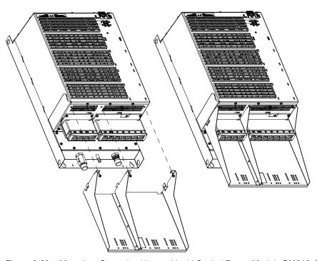
Figure 9-29 Mounting: Screening kit on a Liquid Cooled Power Module PM340, frame size FSF
