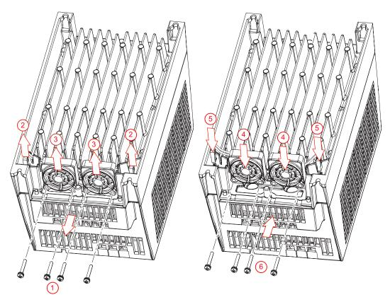
Figure 12-2 PM340 fan replacement, frame size FSB/FSC (0.4 Nm tightening torque)
