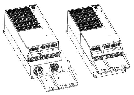
Figure 9-27 Mounting: Screening kit on a Power Module (FSF)
