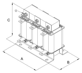
Figure 3-8 Dimension drawing of line reactor, frame size FSF
