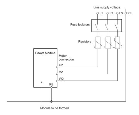
Figure 12-13 Forming circuit for 3-ph AC Power Modules with resistors
