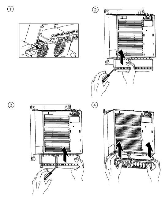
Figure 4-16 Access to the line and motor terminals for Liquid Cooled Power Modules
