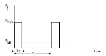
Figure 5-5 Load diagram for the braking resistor, in blocksize format
