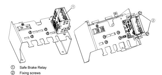
Figure 8-13 Installing the Safe Brake Relay and screening kit (frame sizes FSB / FSC)
