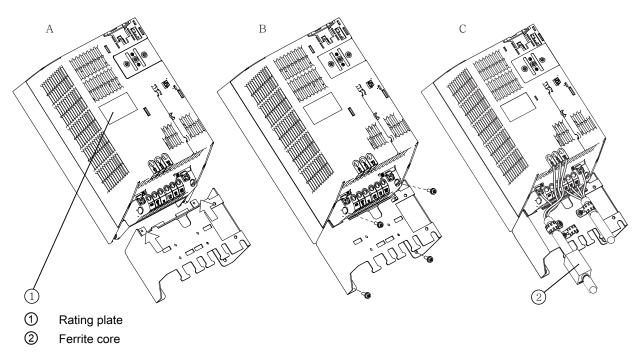
Figure 9-24 Mounting: Screening kit and ferrite core on a Power Module (FSB / FSC)
