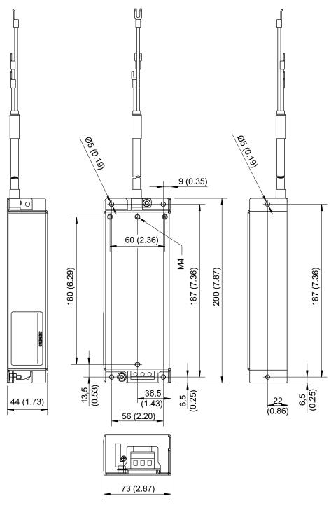
Figure 3-3 Dimension drawing of the line filter, frame size FSA, all data in mm (inches)
