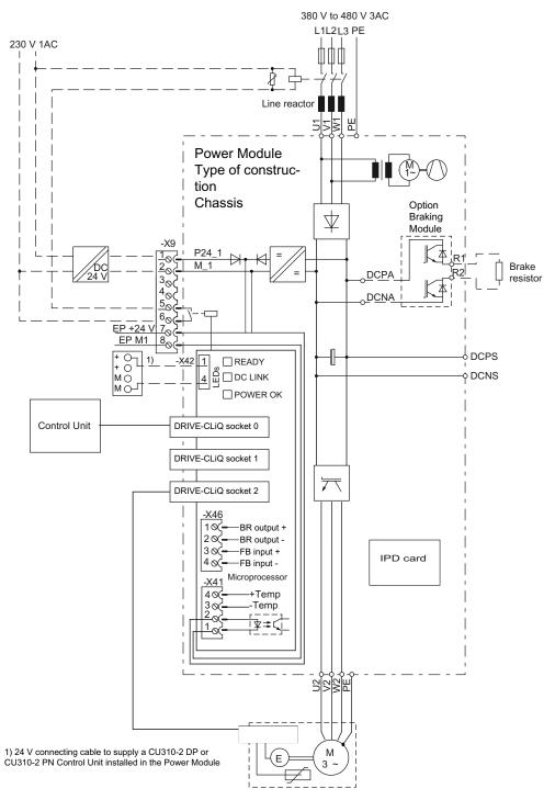
Figure 4-52 Connection example: Power Module chassis
