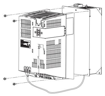
Figure 3-14 Mounting the PM340 with a line reactor, using frame size FSB as an example
