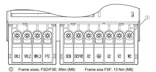
Figure 4-31 PM340 Liquid Cooled: Arrangement of the line and motor terminals (frame sizes FSD to FSF)
