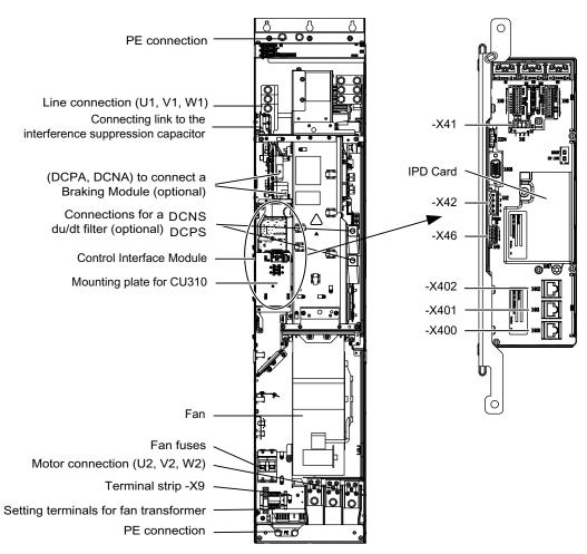
Figure 4-51 Power Module, frame size GX
