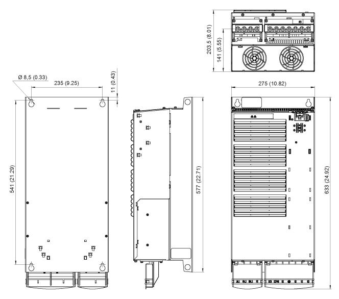
Figure 4-13 Dimension drawing, PM340 Power Module, frame size FSE (with integrated line filter); all dimensions in mm and (inches)
