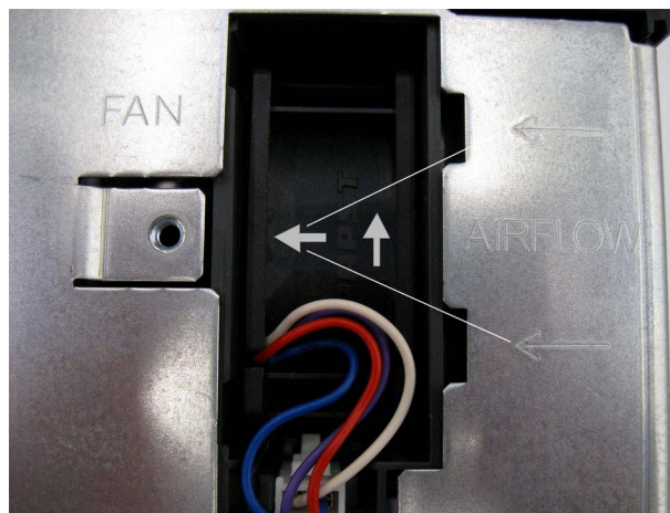
Figure 14-1 Arrows on the fan for the air flow direction
