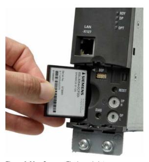
Figure 8-29 CompactFlash card slot
