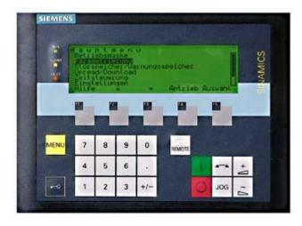
Figure 8-10 AOP30 advanced operator panel (option K08)
