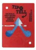
Figure 3-5 Tilt indicator tripped
