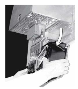
Figure 6-16 Removing the 300mm fan
