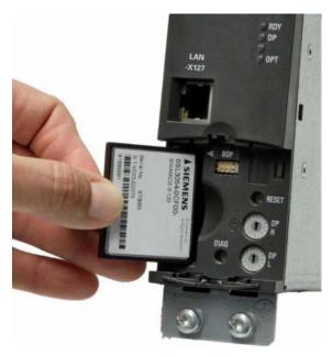
Figure 8-35 CompactFlash card slot
